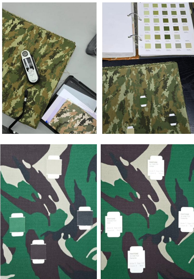
Figures 2, 3, 4, and 5: Color scanning process using a PANTONE® CapSure spectrophotometer and manual matching using PANTONE® TCX color chips. (source: Personal documentation)
