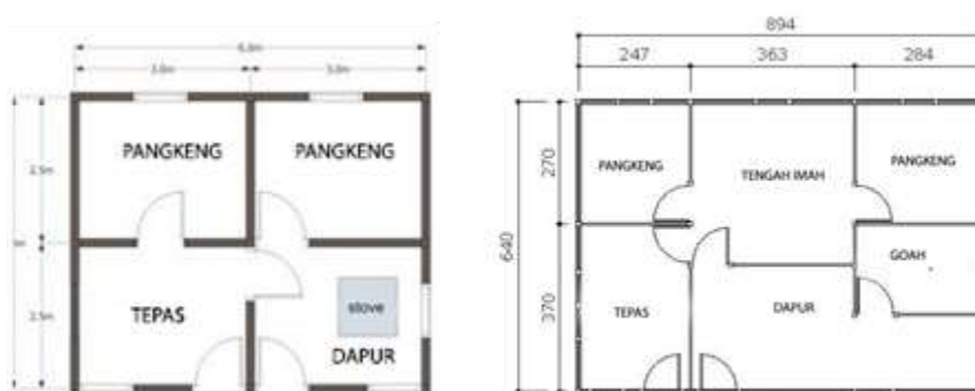
Figure 5. Dimentions differences of Kampung Naga traditional houses Source : MM Sudarwani (2016)
